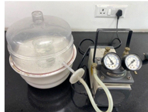
Fig 6 Vacuum Test (-500mmHg) on glued impellers.
