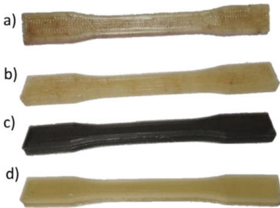
Fig. 7. Composite filament based specimens (a) PLA (90%) + CoF (10%), (b) PLA (90%) + JF (10%), (c) PLA (90%) + CF (10%) and (d) Plain PLA.
