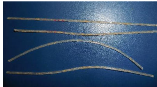
Fig. 10. Samples of PLA(90%) + JF(10%) filament.
