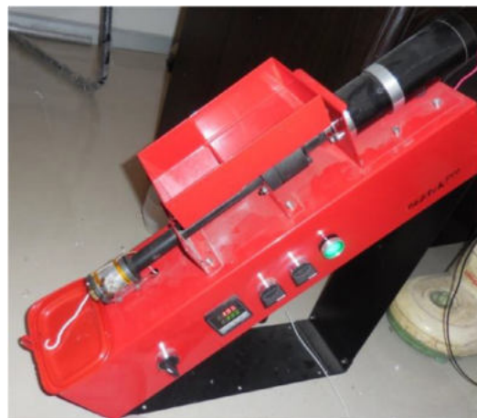
Fig. 1. Experimental raw material filament extrusion.
