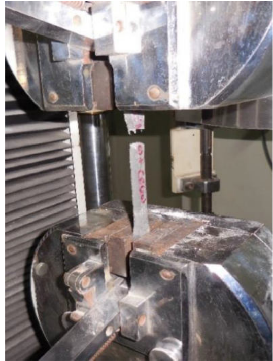
Fig. 9. Brittle Fracture of PLA(90%) + CF(10%) specimen.
