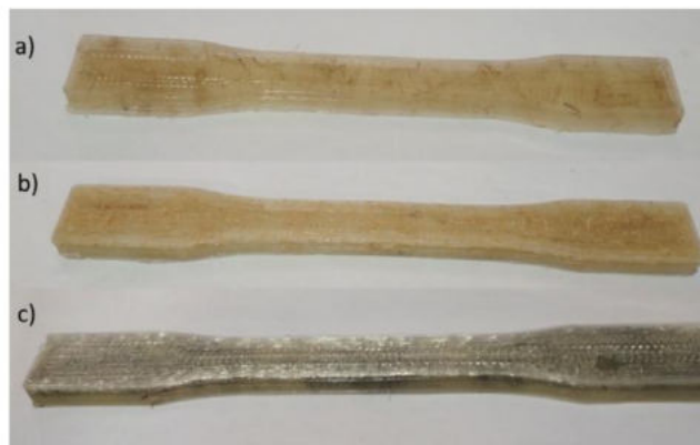
Fig. 8. Sprinkled direct deposition method based specimens (a) PLA (90%) + CoF (10%), (b) PLA (90%) + JF (10%), (c) PLA (90%) + CF (10%).
