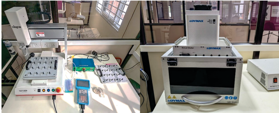
Fig 3 Glue Robot (Left), UV Equipment to Cure the Glue (Right)
